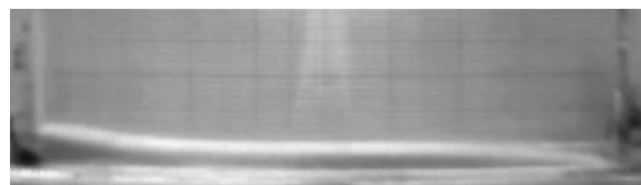
Figure 4. Photograph taken just after vibration of the bed illustrating the occurrence, in this particular case, of surface heaping during the previous vibration process ( \Gamma = 4.4 , \nu = 200 Hz).
